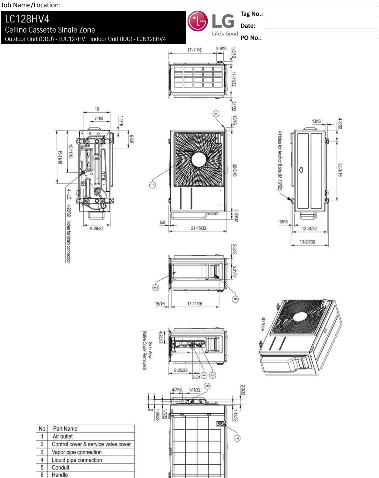
Handle 6 7 Intake air temperature sensor cover
