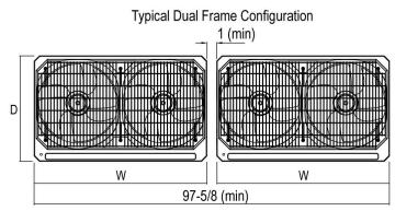
**Note:** Please refer to multi-frame placement information and piping rules in the Multi V 5 Engineering Manual and the Multi V 5 Installation Manual. Minimum spacing between frames is 1 inch.
