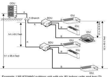
Example: LMU421HHV outdoor unit with six (6) indoor units and two (2) branch distribution units connected. ODU: Outdoor Unit. IDU: Indoor Unit. BDU: Branch Distribution Unit(s). A: Main Pipe. B: Branch Pipe (Branch Distribution Unit[s] to Indoor Unit[s]).
