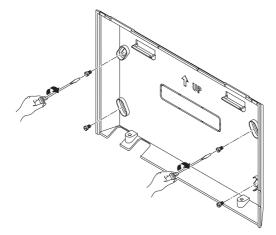
3. Extend the RS485 cable through the top opening of the back panel.
