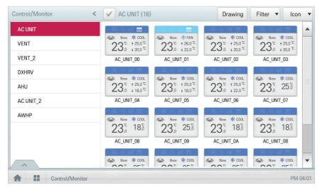
5. To check the control status of the device, touch the [Detail.] button.
