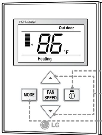
**1** If you want to set the heating operation, press the On/Off button. And press the mode button.
