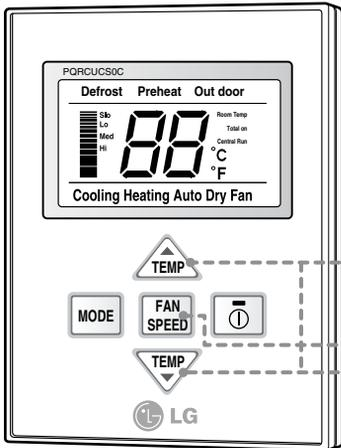
**1** If you want to change the temperature unit as the Celsius or Fahrenheit, press the Temperature control button(▼) and the Fan speed button same time for three seconds to enter the setting Mode.
