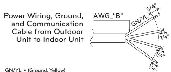
Power Wiring, Ground, and Communication Cable from Outdoor Unit to Indoor Unit
