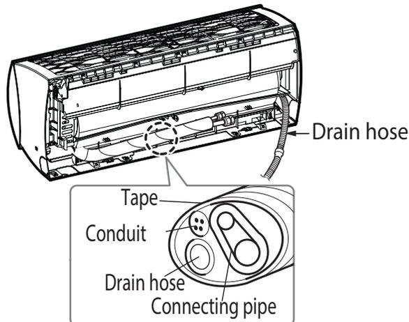
Figure 46: Piping with Insulation Material
