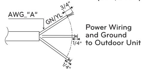
Power Wiring and Ground to Outdoor Unit
