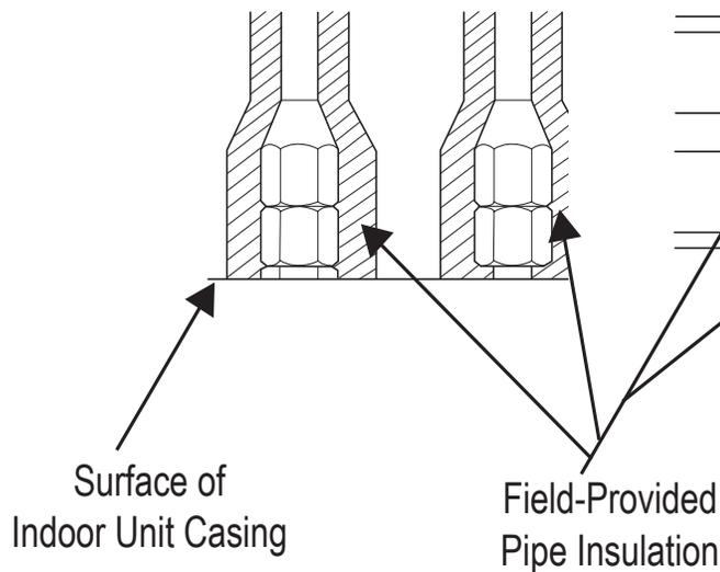
Figure 53: Typical Refrigerant Flare Fitting Insulation Detail
