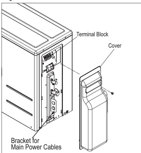
Figure 68: 18k/24k ODU Cover Removal
