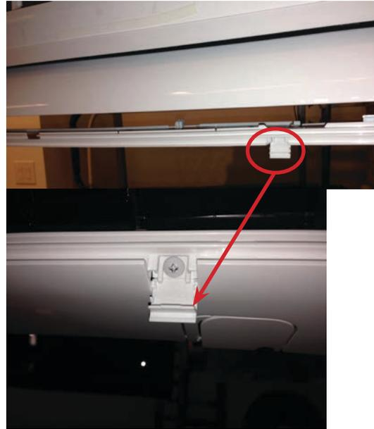
Figure 61: Remove Screws from Bottom Panel
