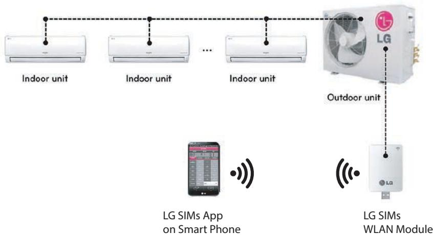
Figure 76: SIMS WLAN Module to Typical DFS System
