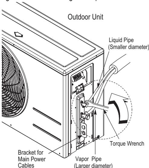
Figure 41: 18k/24k Refrigerant Pipe Connections
