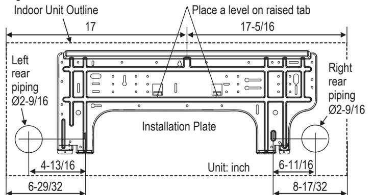
Figure 11: LAN180HYV1 / LAN240HYV1 Installation Plate Dimensions
