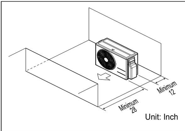
Figure 7: Clearances Where There are Obstacles Above and on Both Air Inlet and Outlet Sides (Obstacle on the Outlet Side is Lower Than the Outdoor Unit)
