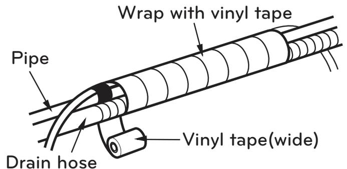
Figure 50: Bundling and Placement at Rear of IDU
