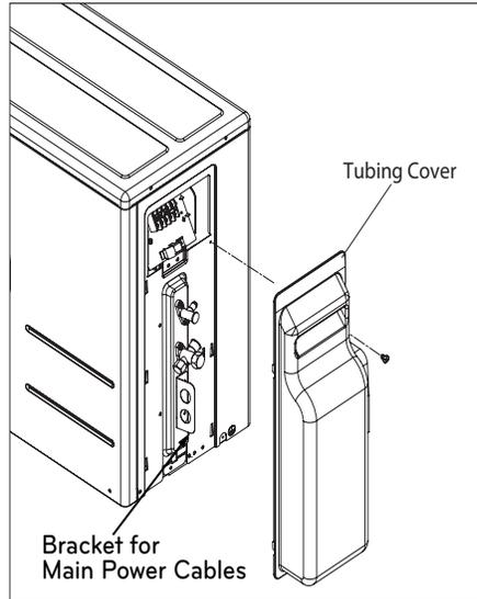
Figure 40: LSU180HSV4 Outdoor Unit Connection Cover Removal.
