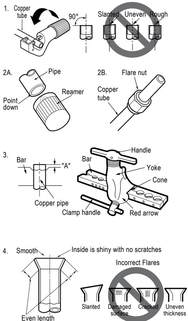
Figure 18: Dimensions of the Flare
