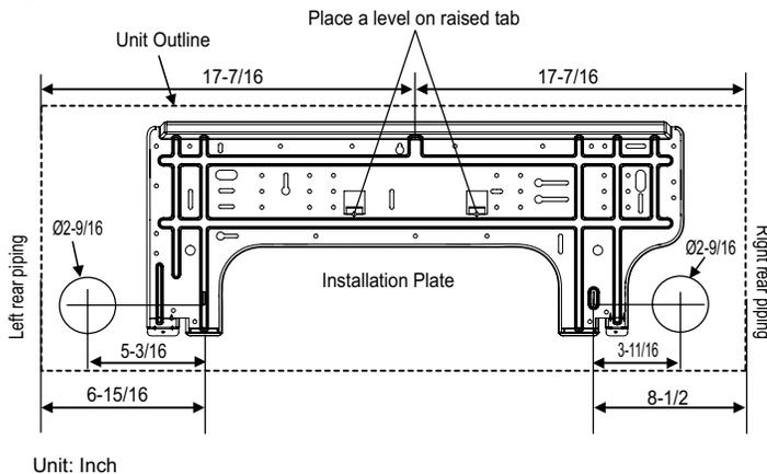
Figure 9: Installation Plate Screws - 090HSV4, 120HSV4
