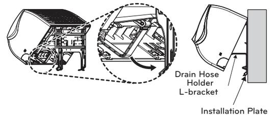
Figure 16: Mounting Bottom of Unit to Installation Plate
