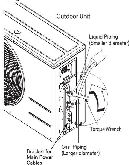
Figure 42: LSU180HSV4 Outdoor Unit Piping Connection.
