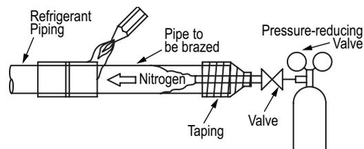
All joints are brazed in the field. Single Zone Art Cool Mirror system refrigeration components contain very small capillary tubes, small orifices, electronic expansion valves, oil separators, and heat exchangers that can easily become blocked. Proper system operation depends on the installer using best practices and utmost care while assembling the piping system.
