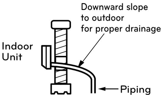
Figure 37: Correct Slope Angle for Drain Hose
