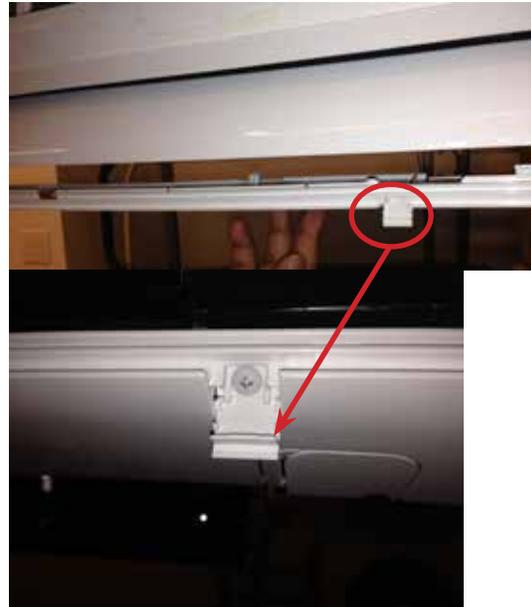
Figure 65: Remove Screws from Bottom Panel
