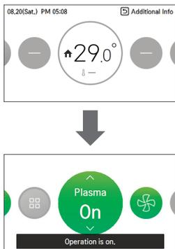
In case of plasma purification single operation, it operates in fan mode / automatic wind state, and the wind direction operated before the plasma purification single operation is turned off.
