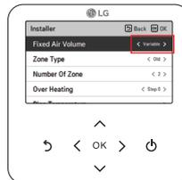
In each detail screen of the menu, as in the box in the left figure, when "<, >" icons are displayed at the same time, you can immediately apply the setting value by pressing [ <, > (left/right) ] button.
