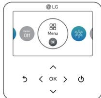
In the menu screen, press [ <, > (left/right) ] button to select the category to set, and press [OK] button to move to the detail screen.
