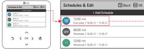
You can check the set timer's operation information (operation On/Off, operation mode, desired temperature, timer time, period, and day of week).
