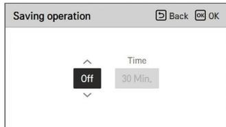
You can select OFF ← → On/Off Power saving ← → Temperature power saving for mode value. You can set the time value when you select On/Off power saving or Temperature power saving.
