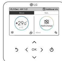
When you control the air conditioner and the ventilation product with one remote controller, the screen is displayed as in the side figure. You can set the air conditioner by pressing [←(left)] button and pressing [OK] button to move to the air conditioner screen.
