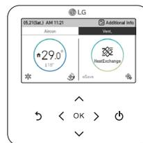
When you control the air conditioner and the ventilation product with one remote controller, the screen is displayed as in the side figure. You can set the ventilation by pressing [→(right)] button and pressing [OK] button to move to the ventilation screen.
