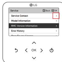
In each detail screen of the menu, as in the box in the left figure, if only ">" icon is displayed, you can move to the detail setting screen by pressing [ > (right) ] or [OK] button.
