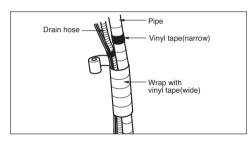
Reroute the pipings and the drain hose across the back of the chassis.
