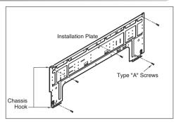
2. Measure the wall and mark the centerline. It is also important to use caution concerning the location of the installation plate. Routing of the wiring to power outlets is through the walls typically. Drilling the hole through the wall for piping connections must be done safely.
