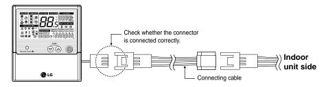
6. When the distance between the wired remote controller and the indoor unit is 10m and above, use the extension cable.
