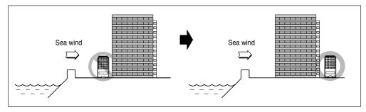
In case, to install the outdoor unit on the seaside, set up a windbreak not to be exposed to the sea wind.
