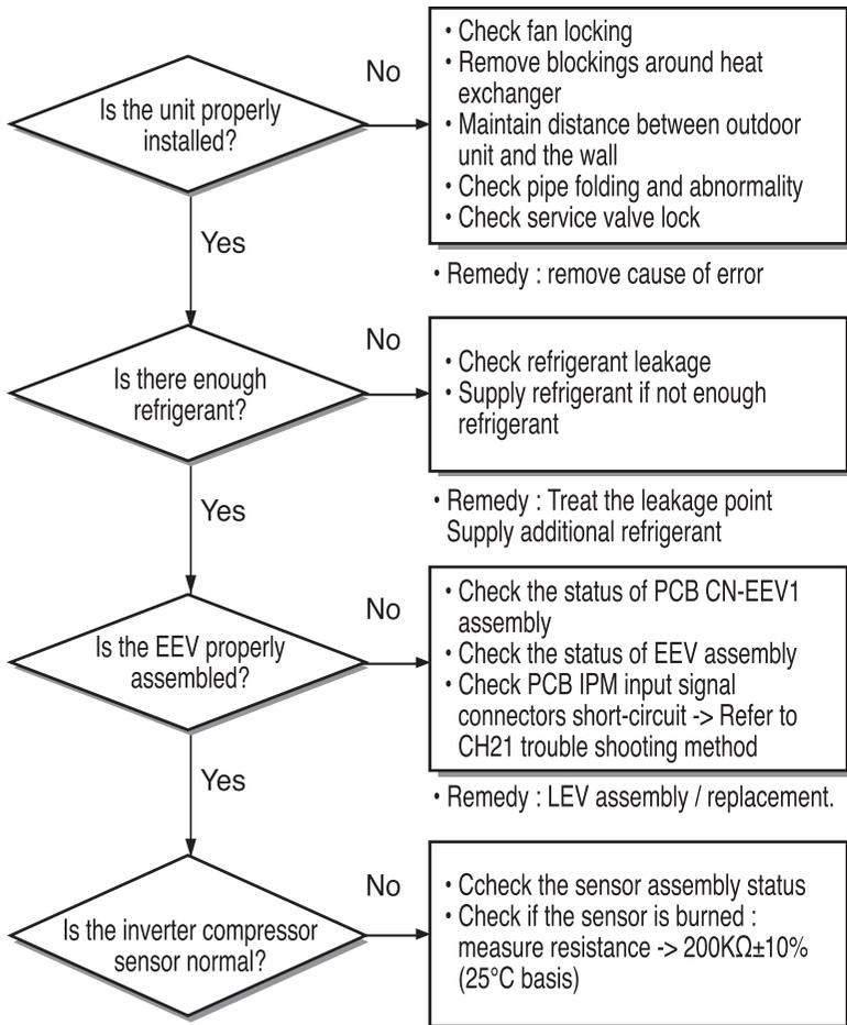
**• Inspecting Inverter Compressor Discharge Sensor**
