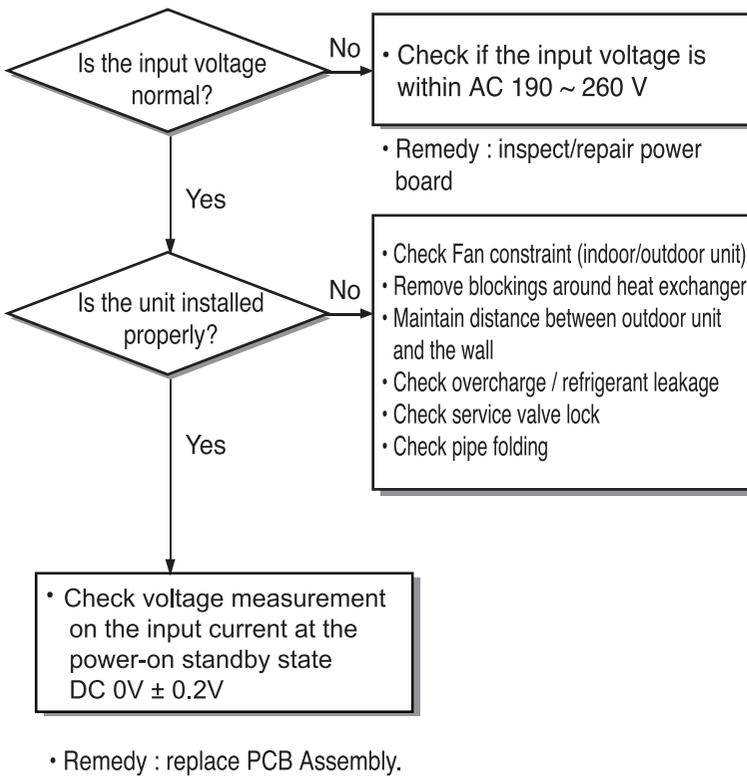
**• Inspecting PCB input current sensing circuit**
