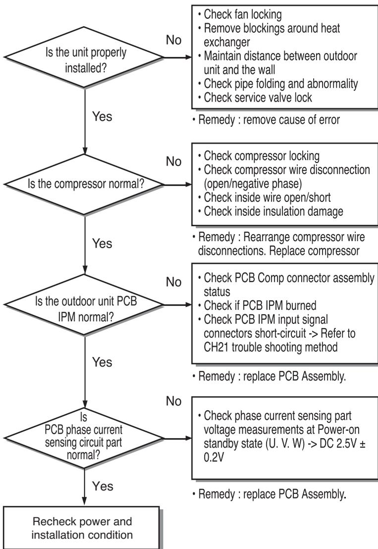
**Inspecting PCB phase current sensing circuit**
