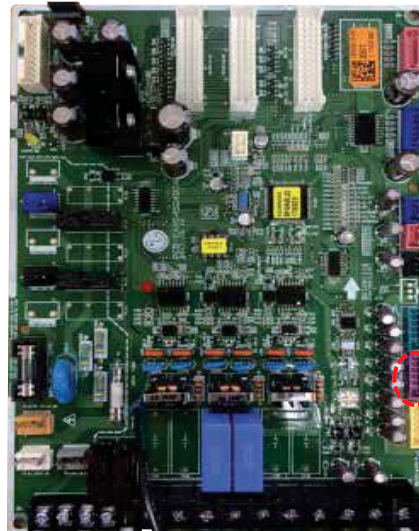
Figure 54: ARUN060GSS4 and ARUB060GSS4 Error No. 41 Checking the Inverter Compressor Discharge Temperature Sensor Resistance.
