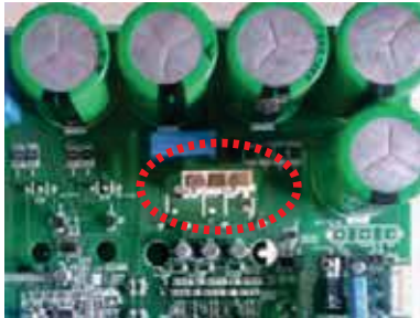
Figure 50: ARUN060GSS4 and ARUB060GSS4 Error No. 29 Compressor Terminal and Wiring Connections.
