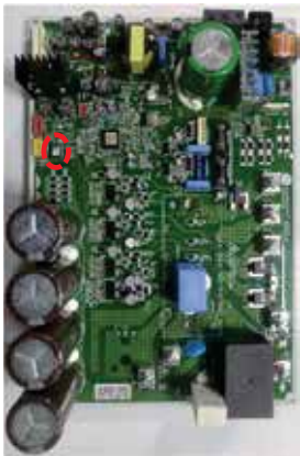
Correct Inverter EEPROM Installation Direction.
