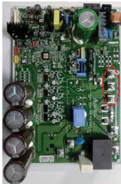
Figure 48: ARUN060GSS4 and ARUB060GSS4 Error No. 22 Compressor Terminal and Wiring Connections.
