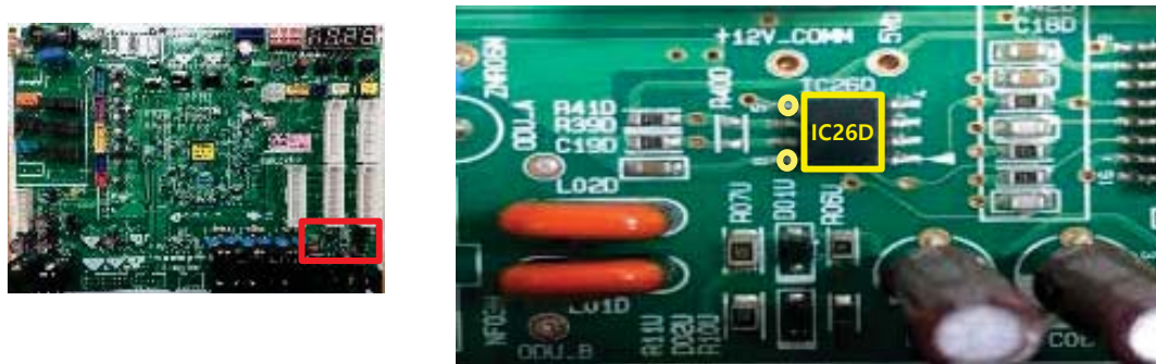
Figure 82: Checking Main PCB (Communication IC).
