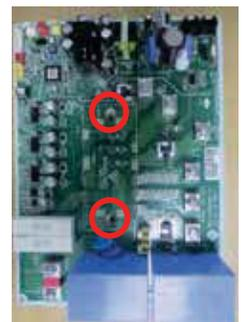
Figure 70: Removing the Inverter PCB.
