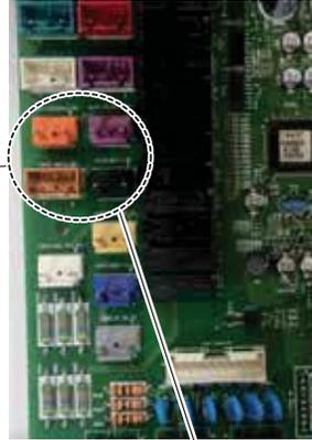
Confirm the four-way valve coil is completely inserted.
