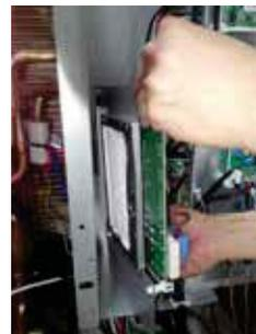
Figure 71: Removing the PCB.
