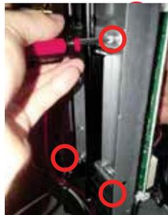
Figure 68: Disconnecting the Compressor and Power Input Wiring.
