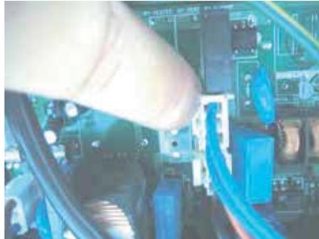
\*\* Indoor PCB Drain Pump Connector
