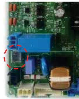
\*\*Check if the high pressure switch connection has shorted out.
