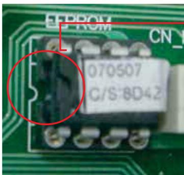
Both the socket opening and the EEPROM opening must be in the same direction.
