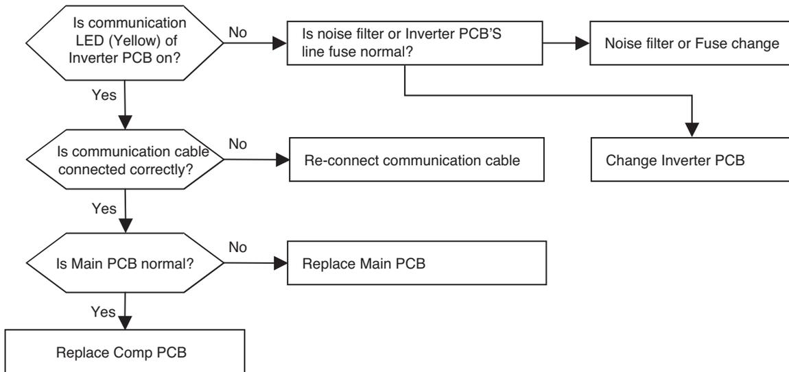
\* The method of checking Main PCB and Inverter 2 PCB (If normal, communication LED blinks)
