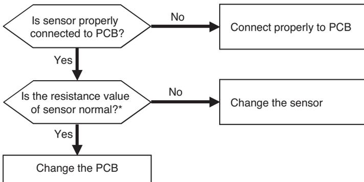
\* In case the value is more than 100 kΩ (open) or less than 100 Ω (short), Error occurs
