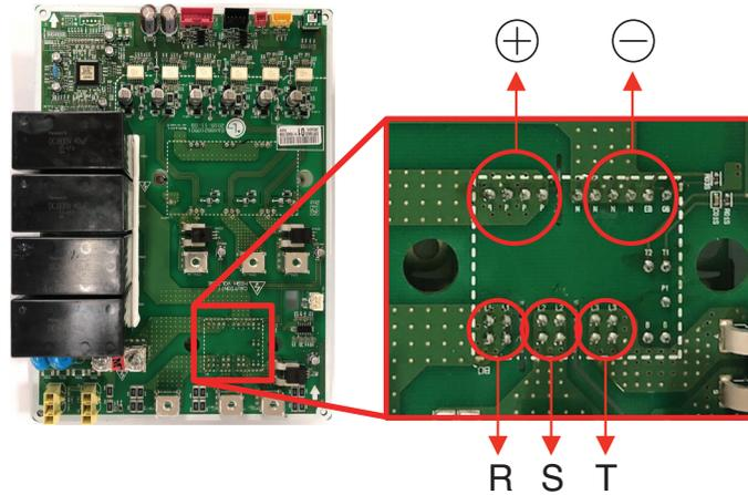
1. Wait until Comp PCB DC voltage gets discharged, after the main power switch off (10 minutes).
