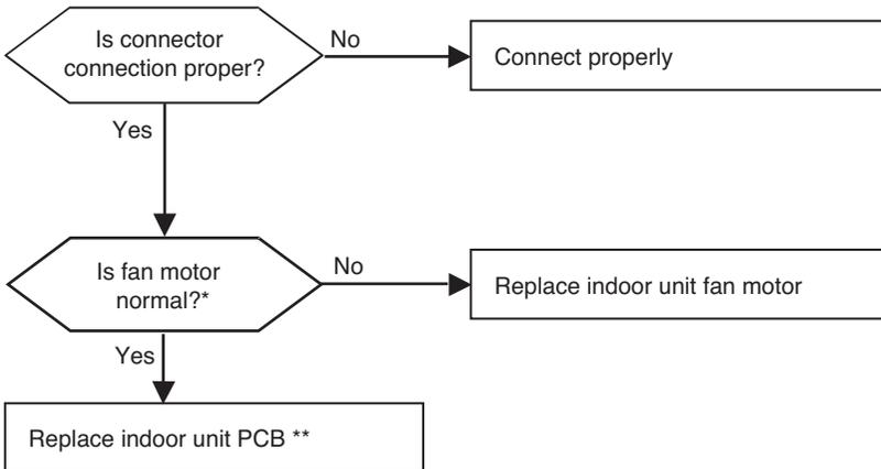
\* It is normal when check hall sensor of indoor fan motor as shown below
