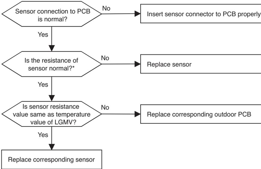
\* Error is generated if the resistance is more than 5 MΩ(open) and less than 2 kΩ (short)
