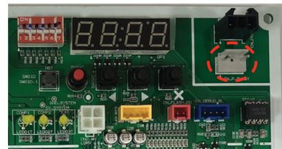
Note 2) Check short with high pressure switch connector
