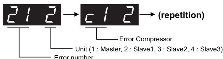
\* Refer to the DX-Ventilation manual for DX-Ventilation error code
