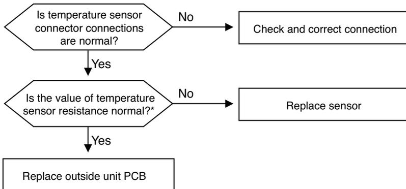
\* Sensor resistance 100 kΩ over (open) or 100 Ω below (short) will generate error
