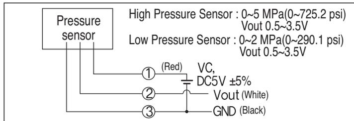
The pressure sensor is composed like the circuit picture shown above. If DC 5V voltage flows on red and black wire, voltage would be made between the white and black wire. The pressure which is equivalent to the pressure output is shown in the table above.
