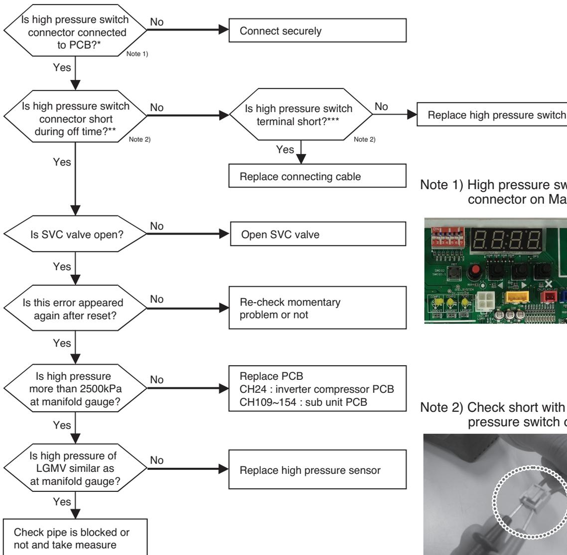
Note 1) High pressure switch connector on Main PCB
