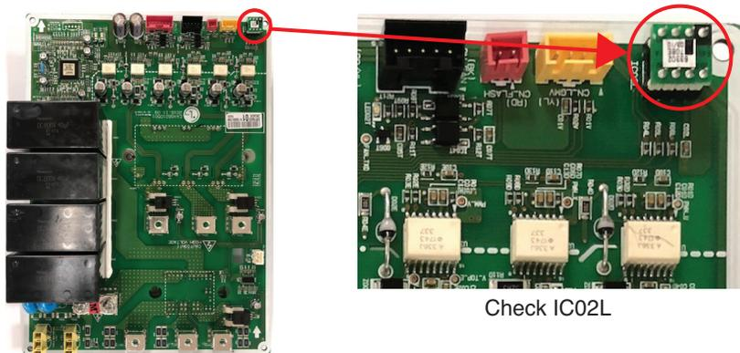
\* Right inserting direction of inverter EEPROM
