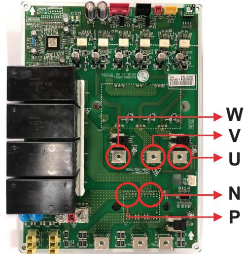
1. Wait until the Inverter PCB DC voltage is discharged after main power off. (10 minutes)
