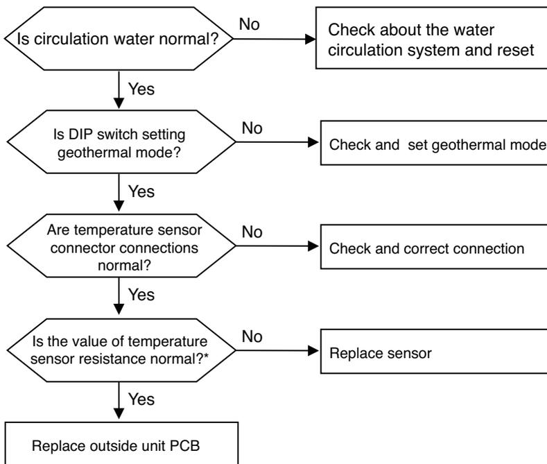
\* Sensor resistance 100 kΩ over (open) or 100 Ω below (short) will generate error
