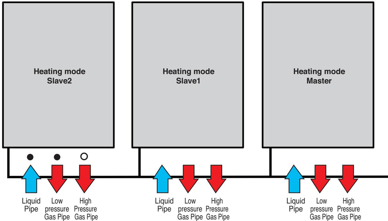
1. Close liquid pipe and low pressure gas pipe of the unit for pump out operation.
