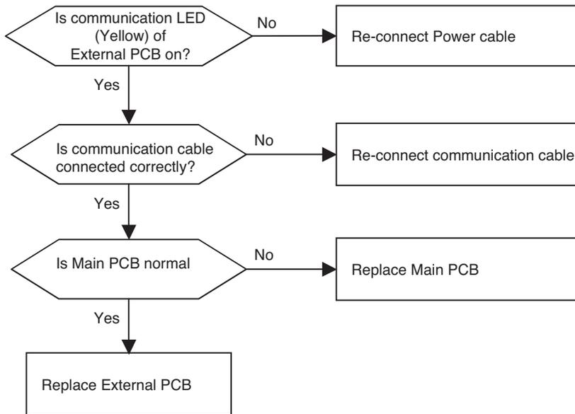
\* The Method of checking Main PCB and External PCB (If normal, communication LED blinks)
