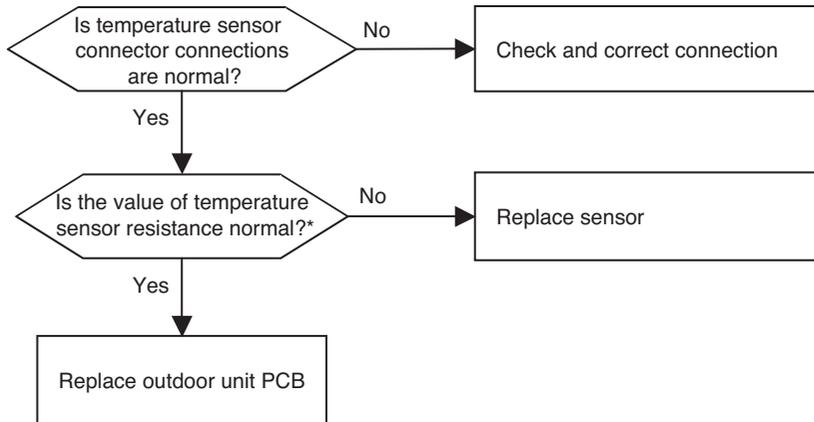
\* Sensor resistance 100 kΩover (open) or 100 Ω below (short) will generate error
