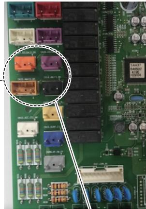
\*\* Confirm the 4way valve coil is inserted to the end
