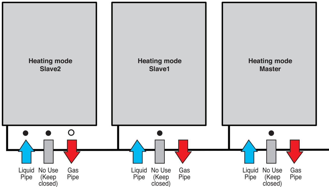
1. Close liquid pipe of the unit for pump out operation.
