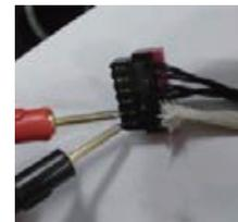
Check the resistance inverter compressor discharge temperature sensor
