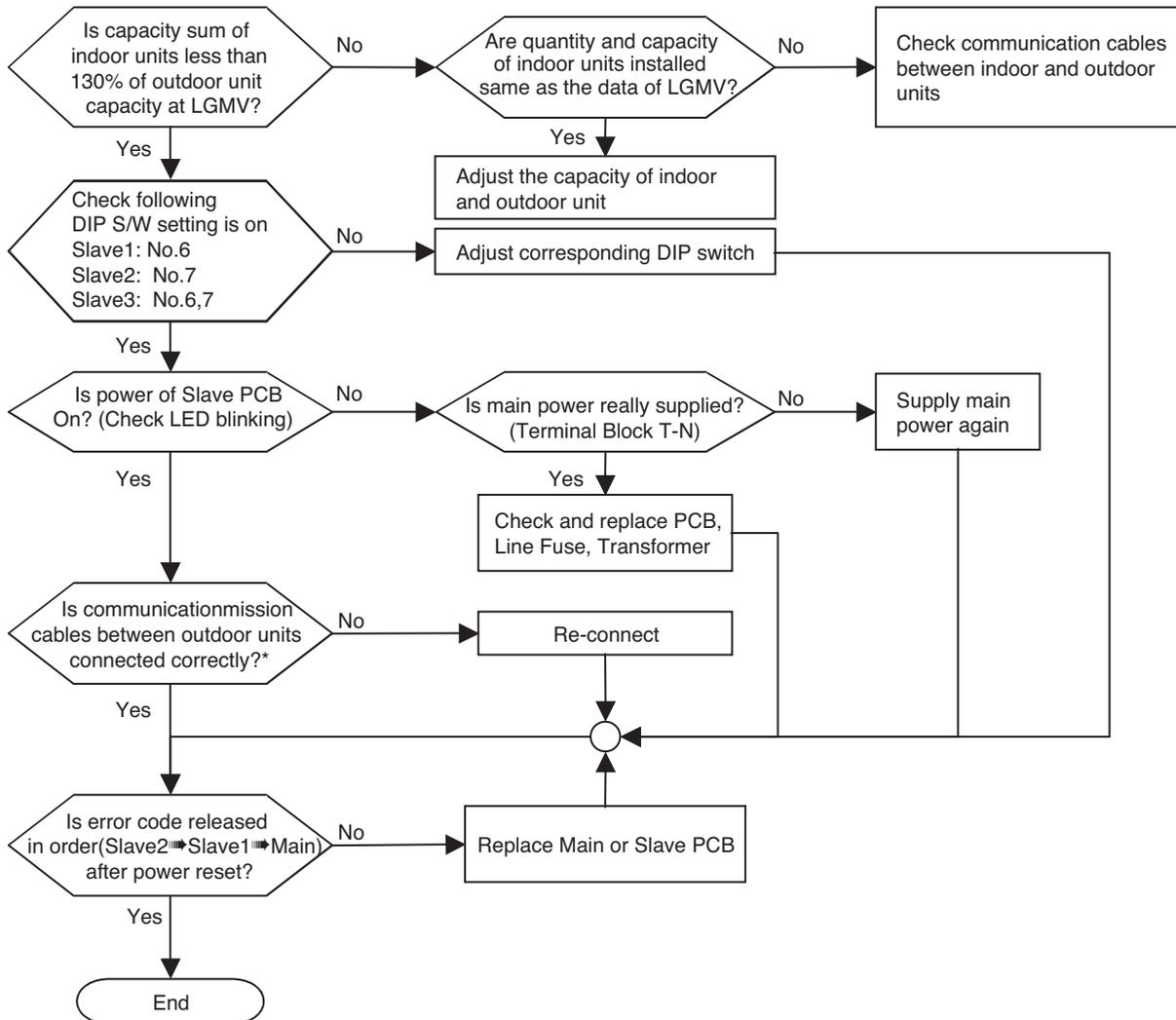
\* In order to check communication cables between outdoor units, check in order as below : PCB connectors → terminal block → communication cables
