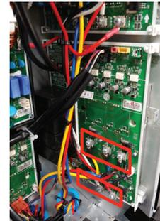
4. Unscrew the middle IGBT mounting screws (2EA)
