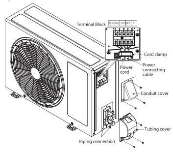
Figure 37: Heat Pump Outdoor Unit Piping Connection
