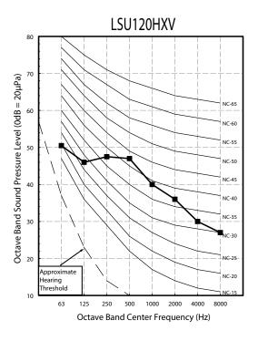
Figure 9: Mega Inverter Sound Measurement
