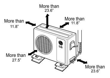
When placing the outdoor unit near a fence, wall or other large obstacle, observe the clearance requirements as shown in Figure 27. This clearance ensures that heat radiation from the condenser is not restricted around the unit.
