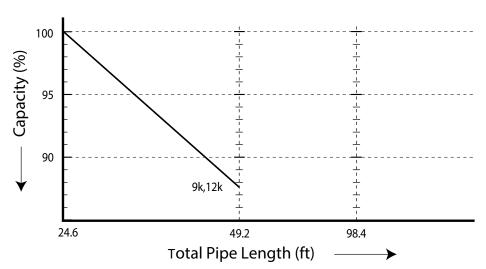
Figure 20: Heating Capacity Coefficient Factor for LS090HXV/LS120HXV
