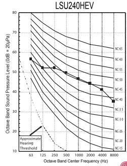
Figure 6: Mega 115V Inverter Sound Measurement
