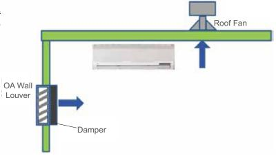
Figure 23: Unconditioned Outdoor Air (Non-Ducted)
