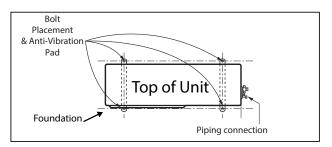
Figure 24: Single Zone Mega Inverter Outdoor Unit—Mounting Methods
