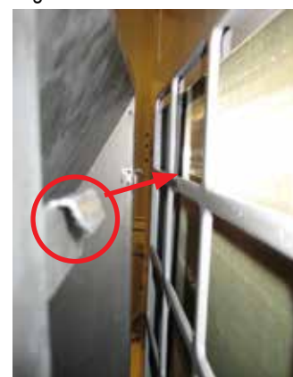
Figure 20: Close up of Wind Baffle Hangers and Where to Attach Them.
