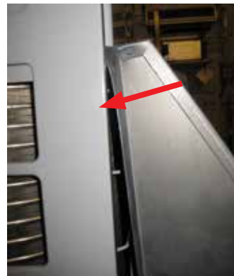
Figure 24: Top Edge of the Rear Wind Baffle Inserted.
