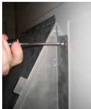
Figure 29: Attaching the Front Wind Baffle.
