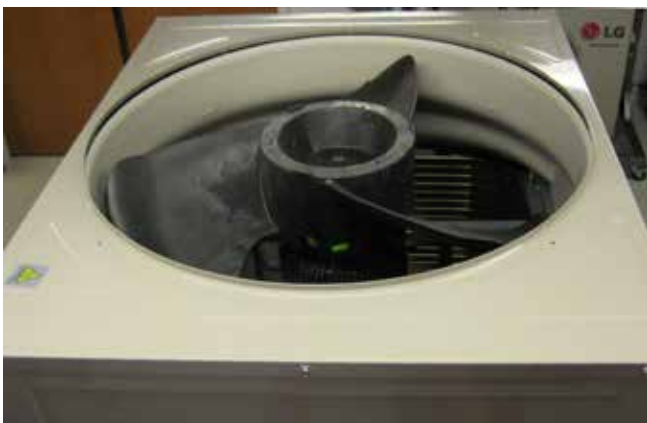
Figure 14: Top of Outdoor Unit with Fan Guard Removed.
