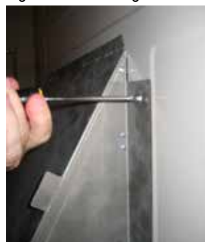
Figure 21: Attaching the Side Wind Baffle.
