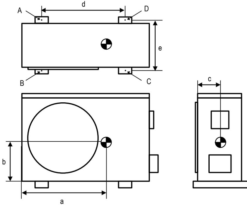
Table 5: Center of Gravity and Corner Weight Dimensions.
