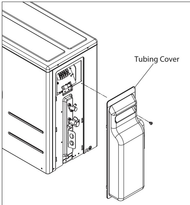
Figure 22: Heat Pump Outdoor Unit Piping Connection
