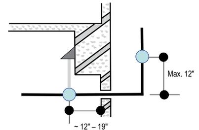
Figure 17: Pipe Support at Indoor Unit.
