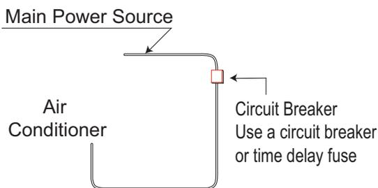
Figure 26: LSN243HLV/LSU243HLV, LSN303HLV/LSU303HLV, LSN363HLV/LSU363HLV Outdoor Unit Electrical Connection.
