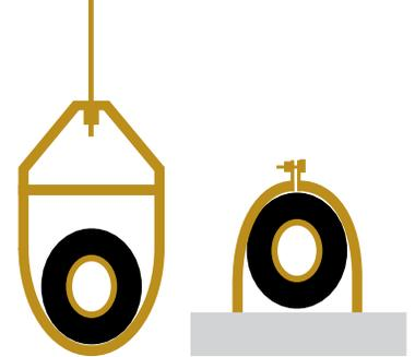
Figure 16: Typical Pipe Support Location—Change in Pipe Direction.
