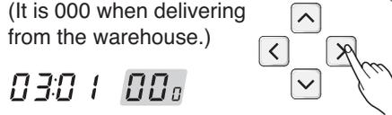
**5** Press button to setup ESP value.
