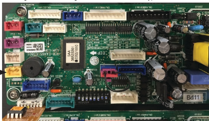
Figure 5: Connecting the Button Sensor to a Typical IDU PCB
