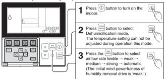
In rainy season or high humidity climate, it is possible to operate simultaneously dehumidifier and cooling mode to remove humidity effectively.
