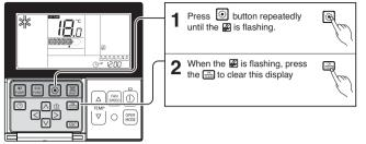
When filter is covered by dust, it will reduce cooling/heating efficiency and accumulate more electric power. Therefore, do clean the filter whenever cleaning time is expired.
