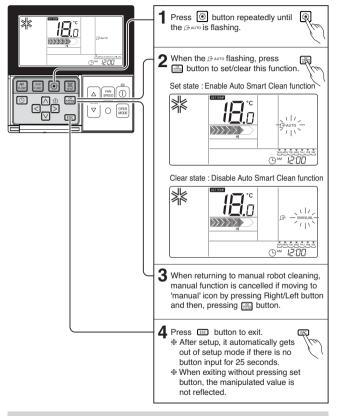
Robot cleaning function is an additional function of the product and might not be operated at the
