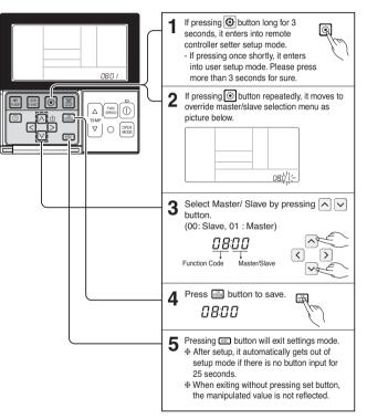
\* Override master/slave selection function is possible to use only when it is connected to the succeeding models of Multi-V 7 series.
