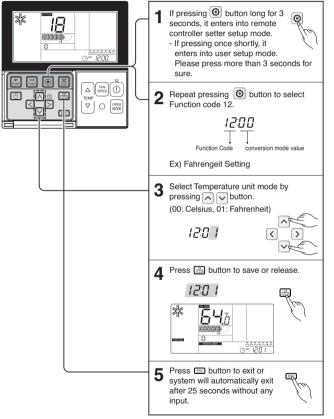
\* Whenever press v button in Fahrenheit mode, the temperature will increase/drop 2 degrees.
