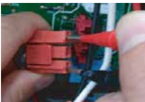
Measure Fan Motor Resistance Between Each Phase.
