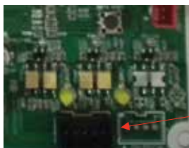
15V Input Power on Inverter PCB.
