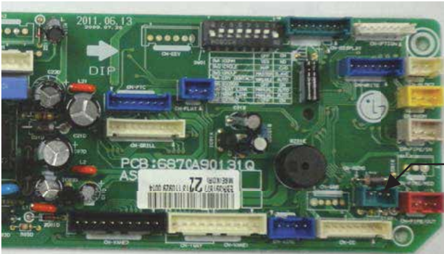
CN-REMO: Remote controller connection ※ The PCB can differ from model to model.
