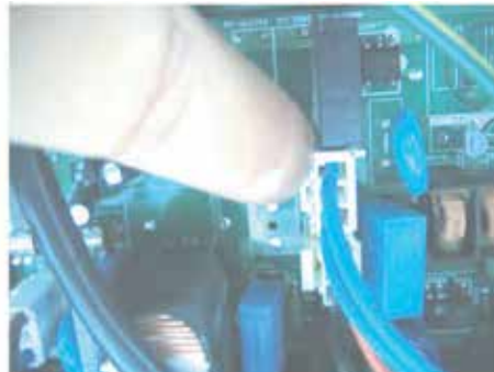
*** Indoor PCB drain pump connector (Check input of 220V) (Marked as CN-DPUMP )
