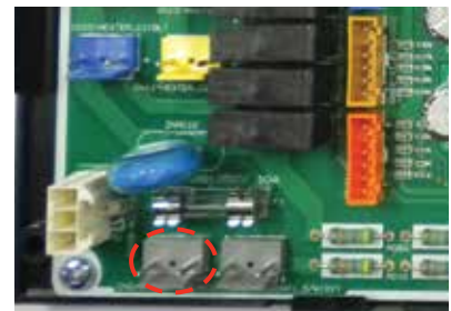
Check if high pressure switch connector has shorted out
