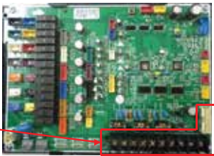
Communication Component in External PCB.
