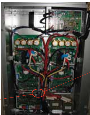
15V Input Power Wiring Connections.
