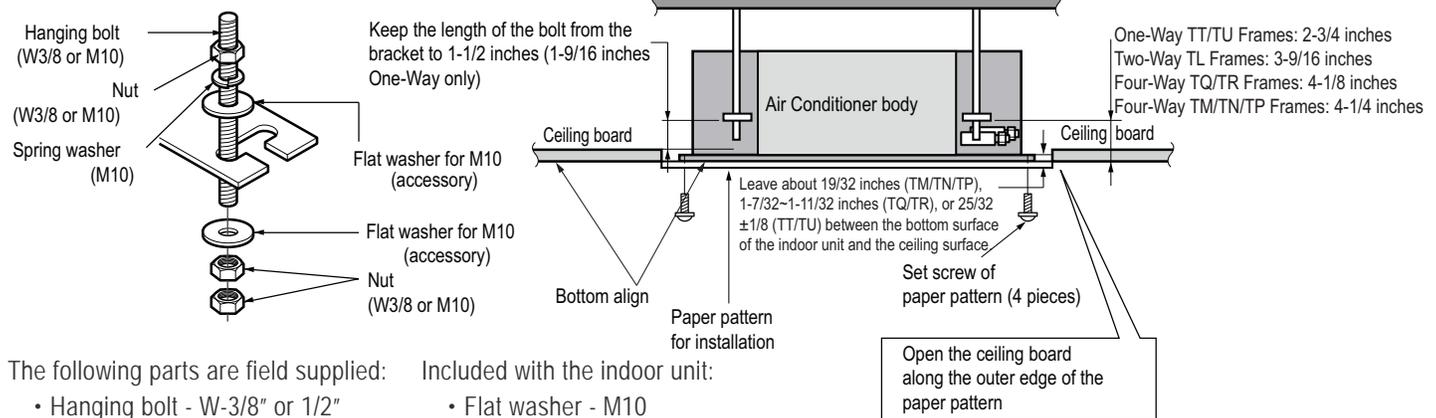
The following parts are field supplied: Included with the indoor unit:
