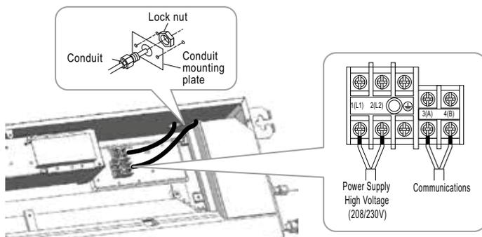
Figure 112: Location of Power Wiring / Communications Cable Terminals in the Two-Way Ceiling-Cassette Indoor Unit.
