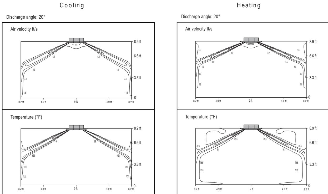
The standard setup height is 8.9 ft. The charts above show the measurement distribution at the ceiling height of 8.9 ft with a high fan operating mode.
