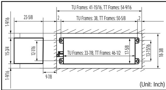
Figure 102: Ceiling Opening / Hanging Bolt Locations for Two-Way Ceiling Cassette Indoor Units.
