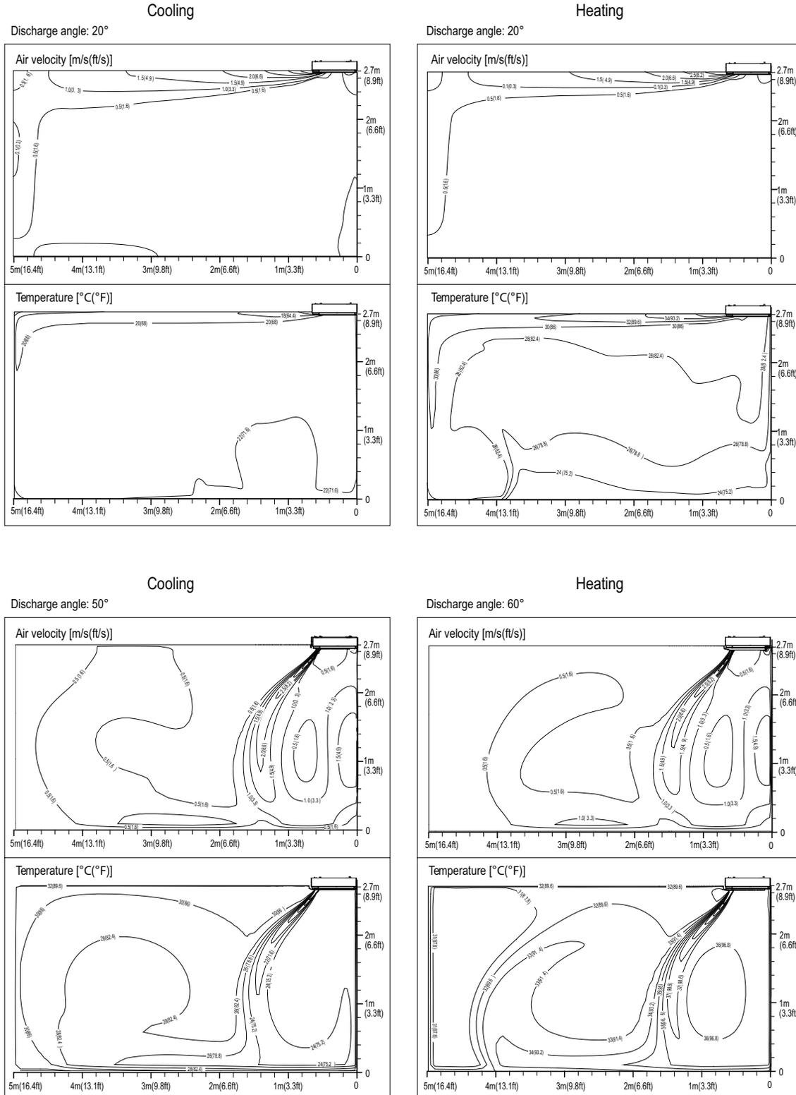
The standard setup height is 8.9 ft. The charts above show the measurement distribution at the ceiling height of 8.9 ft with a high fan operating mode.
