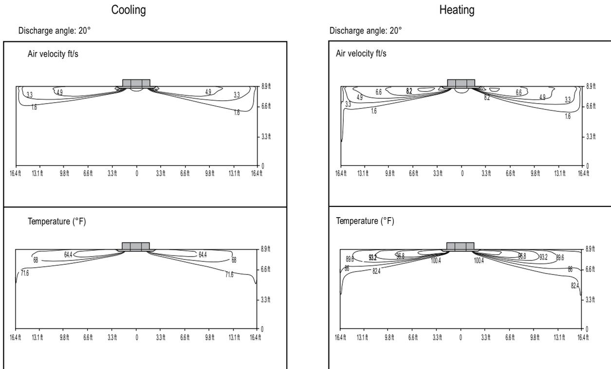
The standard setup height is 8.9 ft. The charts above show the measurement distribution at the ceiling height of 8.9 ft with a high fan operating mode.
