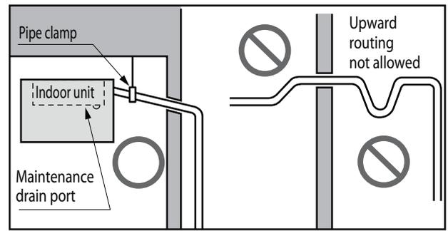
Figure 109: Properly Insulating the Drainage Piping.
