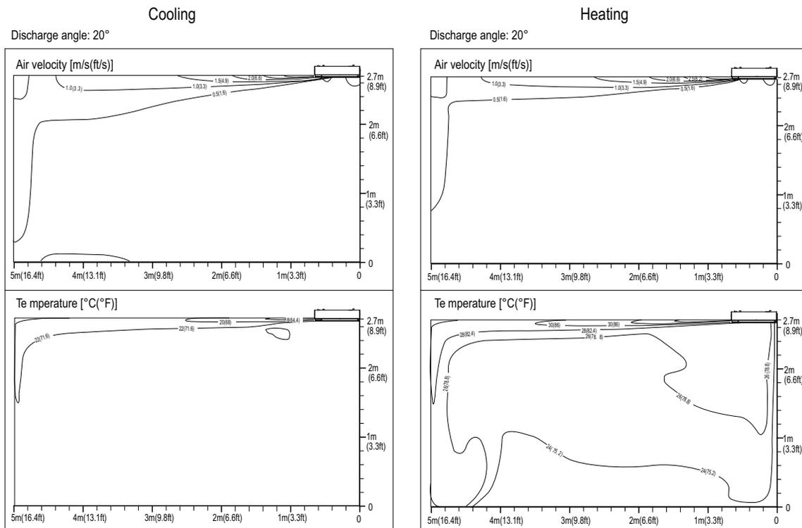
The standard setup height is 8.9 ft. The charts above show the measurement distribution at the ceiling height of 8.9 ft with a high fan operating mode.
