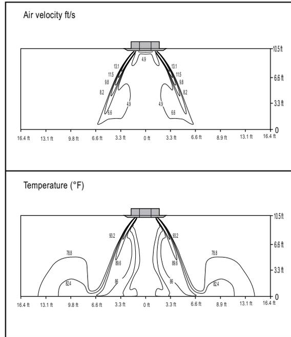
The standard setup height is 8.9 ft. The charts above show the measurement distribution at the ceiling height of 8.9 ft with a high fan operating mode.
