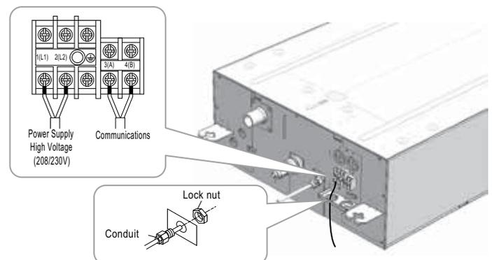
Figure 113: Location of Power Wiring / Communications Cable Terminals in the Four-Way Ceiling-Cassette Indoor Unit.
