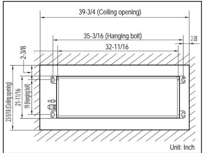
Figure 103: Ceiling Opening / Hanging Bolt Locations for Four-Way Ceiling Cassette Indoor Units.
