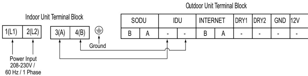
Figure 115: Terminal Block in the Two-Way Ceiling-Cassette Indoor Unit.
