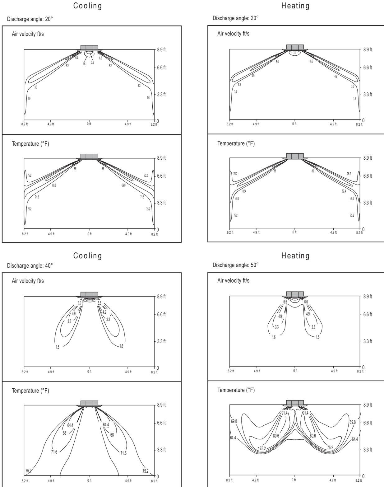
The standard setup height is 8.9 ft. The charts above show the measurement distribution at the ceiling height of 8.9 ft with a high fan operating mode.
