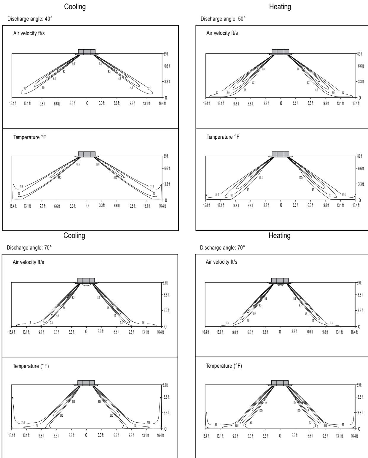
The standard setup height is 8.9 ft. The charts above show the measurement distribution at the ceiling height of 8.9 ft with a high fan operating mode.
