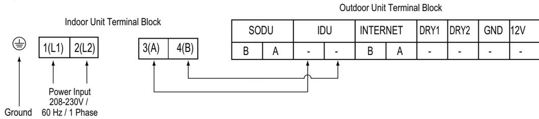
Figure 116: Terminal Block in the Four-Way Ceiling-Cassette Indoor Units.
