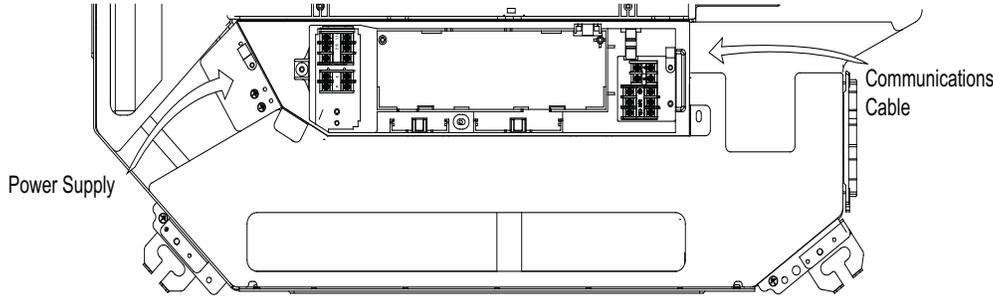
Figure 114: Terminal Block in the One-Way Ceiling-Cassette Indoor Unit.
