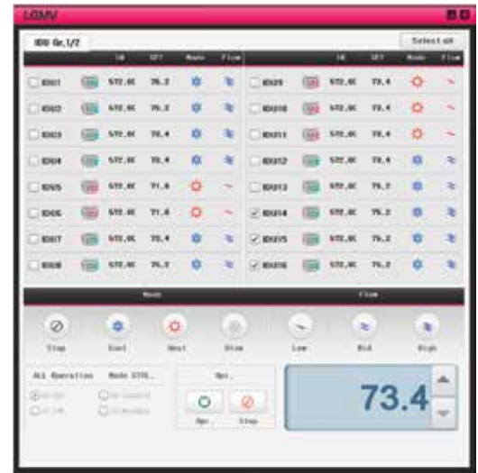
MV Control Indoor Units Screen.
